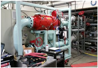
Figure 9. ORC under test at the Calnetix ORC Test Facility.
