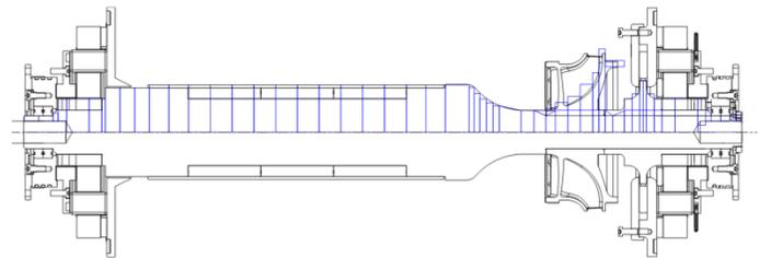
**Figure 5.** Rotordynamic model of IPM rotor.
