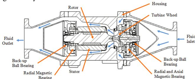
**Figure 4.** IPM cross-section.
