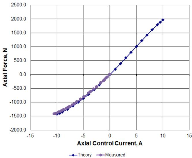
Figure 8. Axial force vs. current – measured vs. theory.
