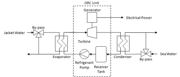
Figure 3. ORC system diagram.
