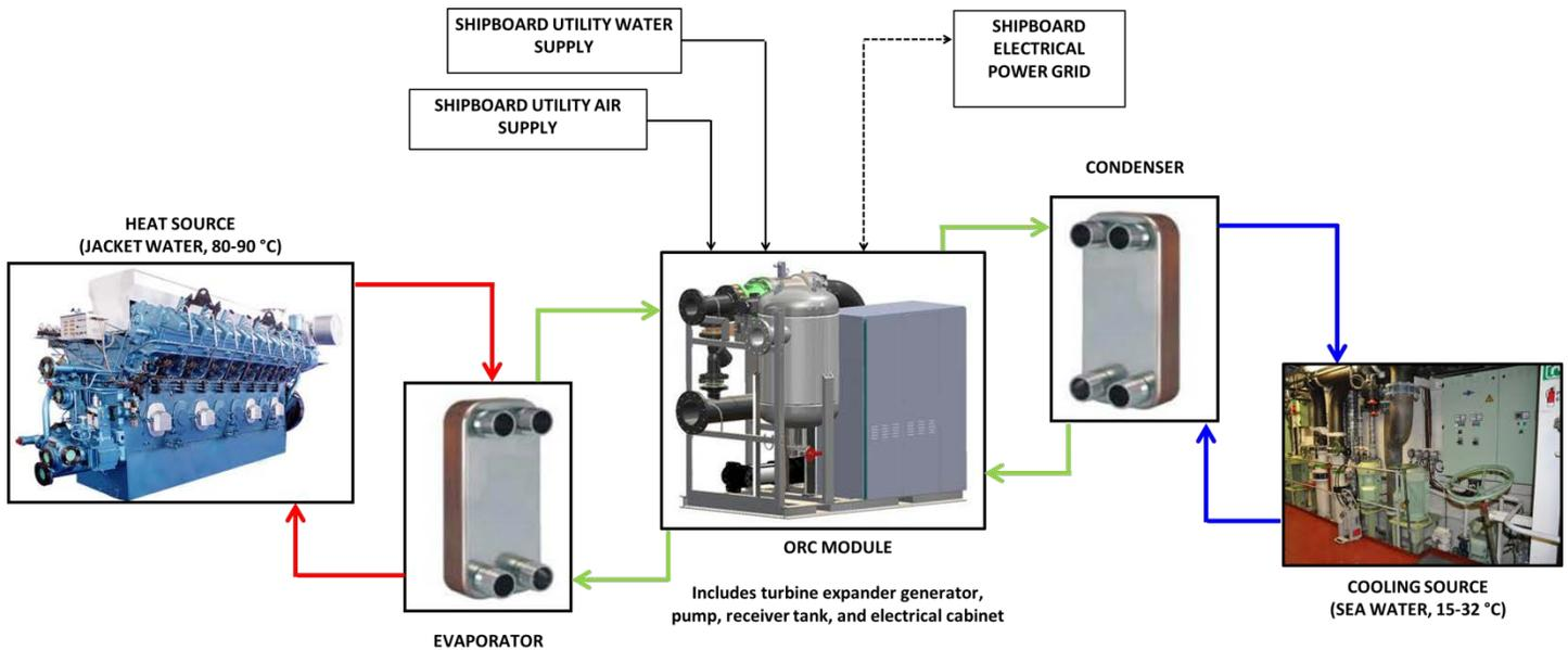
**Figure 1.** ORC system flow and ship interfaces.
