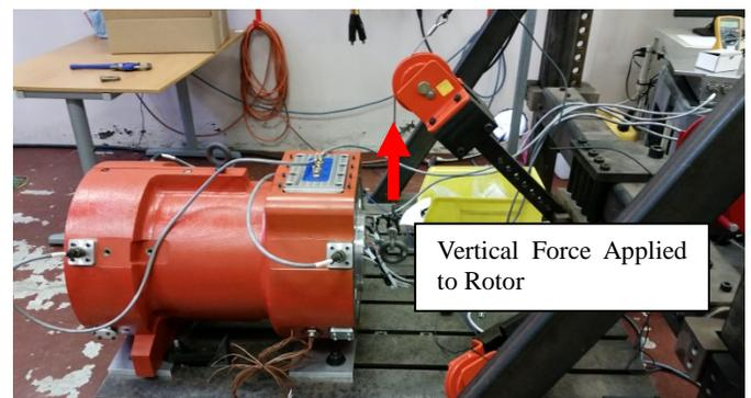
**Figure 7.** IPM under magnetic bearing load testing.
