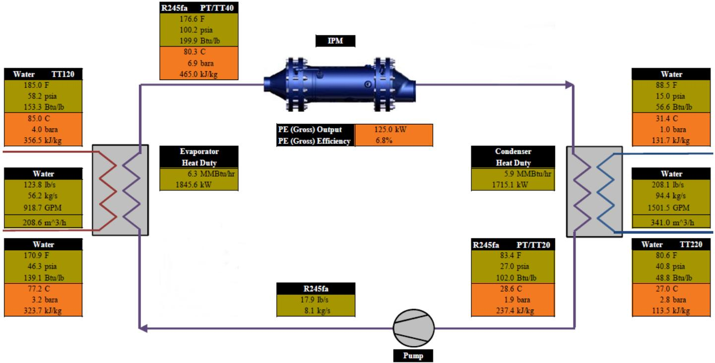
Figure 2. ORC process flow diagram.
