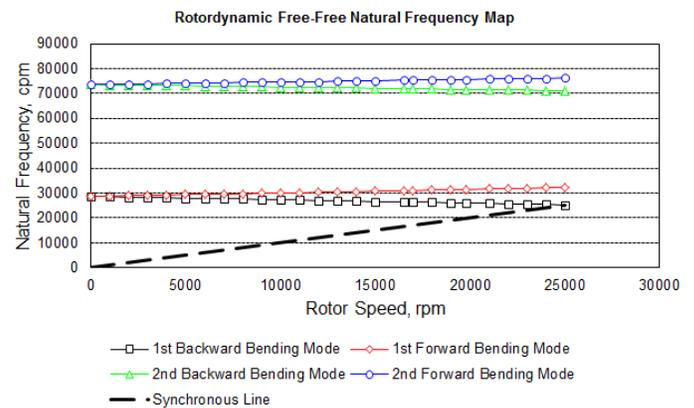
**Figure 6.** Free-free natural frequency map of IPM rotor.
